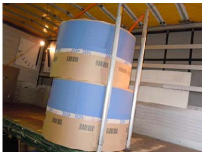
7b. Inclination test for determination of the friction between the reels
