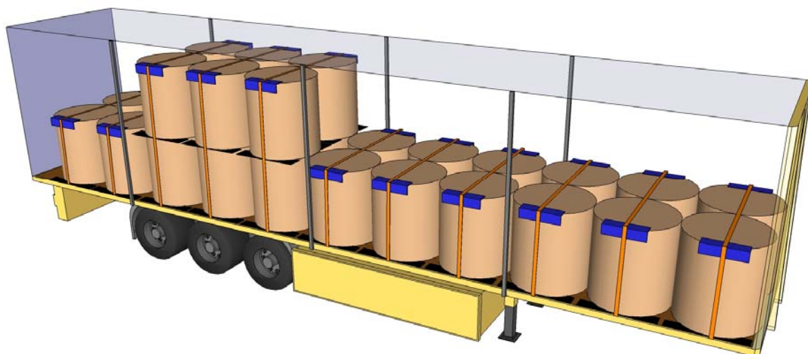
Figure 46. Curtainsider with headboard and rear wall, with rubber put underneath the reels
