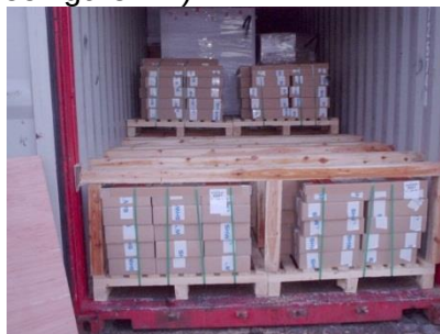
Figure 7.2 Timber temporary floor
