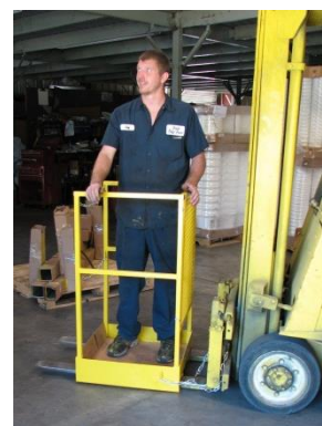
Figure 5.15 Mobile work station
