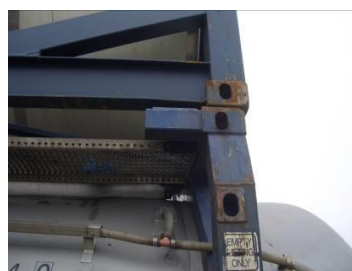
Figure 4.9 Step back with secondary side lift aperture
