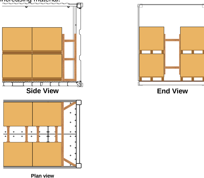
Figure 7.32 Blocking in a strong boundary CTU
