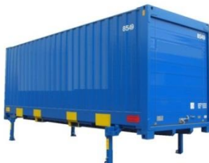
Figure 5.6 Swap body landed on support legs
