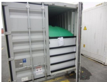
Figure 7.51 Container fitted with flexitank
