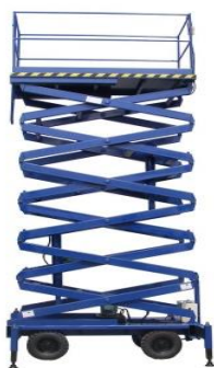
Figure 5.13 Mobile work platform
