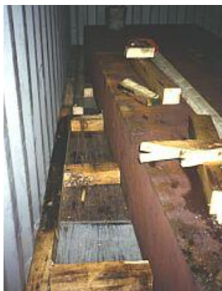
Figure 7.45 Transverse blocking of steel slab
