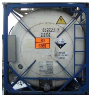
Figure 8.2 Partial frame ladder
