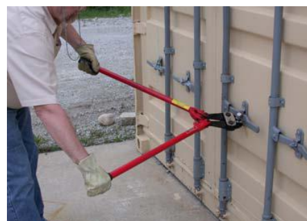
Figure 5.11 Cutting the seal
