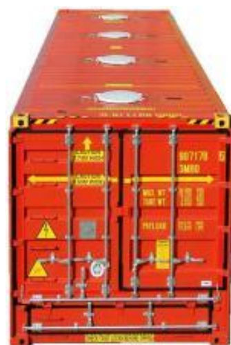
Figure 3.42 30-foot dry bulk box container
