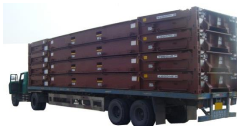
Figure 3.52 – Stack of 40-foot folding end flatracks
